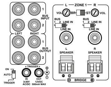
BUS 1 (will play source connected to the BUS 1 input), BUS 2 (will play source connected to the BUS 2 input) or LINE IN (will play source connected to that channel's LINE IN).
